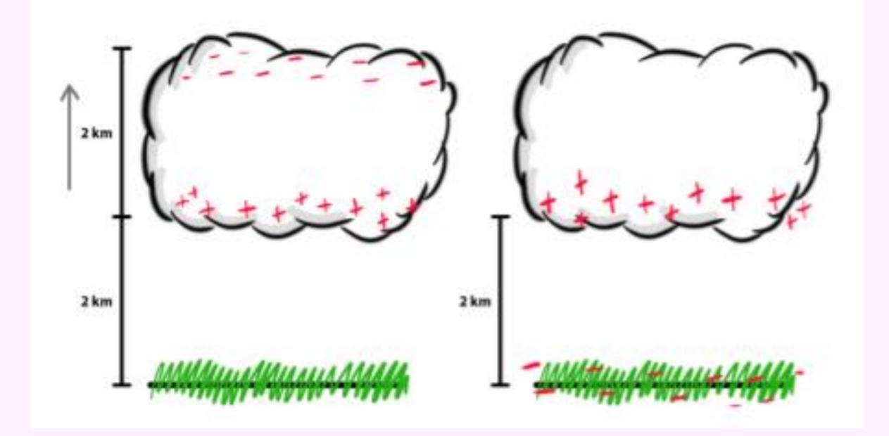
The simple parallel plate capacitor model for our CORSIKA simulations. This project creates Monte Carlo simulations using the Cosmic Ray Simulations for Kascade (CORSIKA). Electric fields ranged between -2000 to 2000 V/cm, using two different types of models: intracloud and cloud-to-ground. Each model is 2km wide, ranging from 3.4 - 5.4km and 1.4 - 3.4km respectively.
