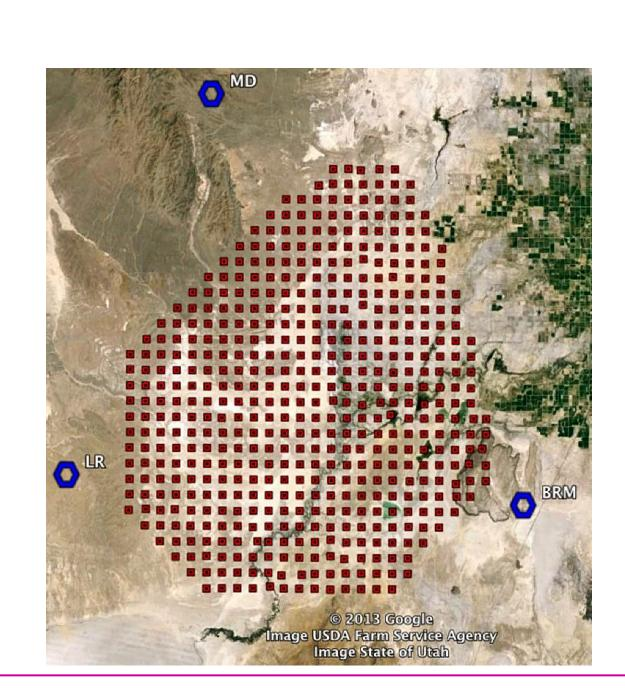
This is the Telescope Array Surface Detector (TASD. Located in Southwestern Utah, the TASD covers a 1.2 km grid. The red filled dots represent the 507 SD scintillators, which are plastic and sensitive to charged particles. The Blue Hexagons indicate the fluorescence detector. The northernmost fluorescence detector is called Middle Drum while the southern fluorescence detectors are referred to as Black Rock Mesa and Long Ridge.
