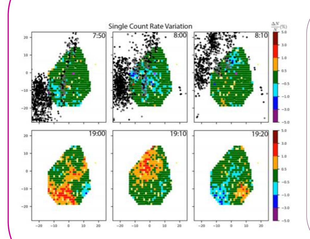
Evolution of Intensity Change over time. These images represent changes in the single count rate change (ΔN/N) in storm data from over the TASD. This storm is from September 27, 2014.
